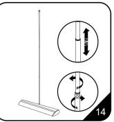
14. Draw out the upper of the telescopic pole to adjust the height to suitable level, then circumgyrate to firm it.
