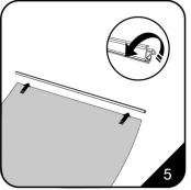
5. Open the snap bar then insert the top edge of the graphic.
