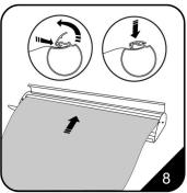
8. Open the roller's lid, slide the bottom edge of the graphic under the lid. Close the roller's lip to secure the graphic.
