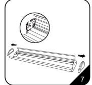
7. Release cover screw, then open the base unit cover
