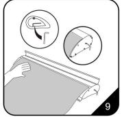
9. Activate the spring tension by removing the Allen Key. Pull the Allen Key while holding on the the attached graphic. Save the key in the side cover.
