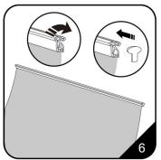
6. Close the snap bar lips to secure the graphic. Finish the top by r e-attaching the end caps.
